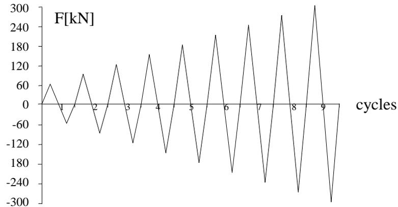
Figure 6: Horizontal loading pattern
