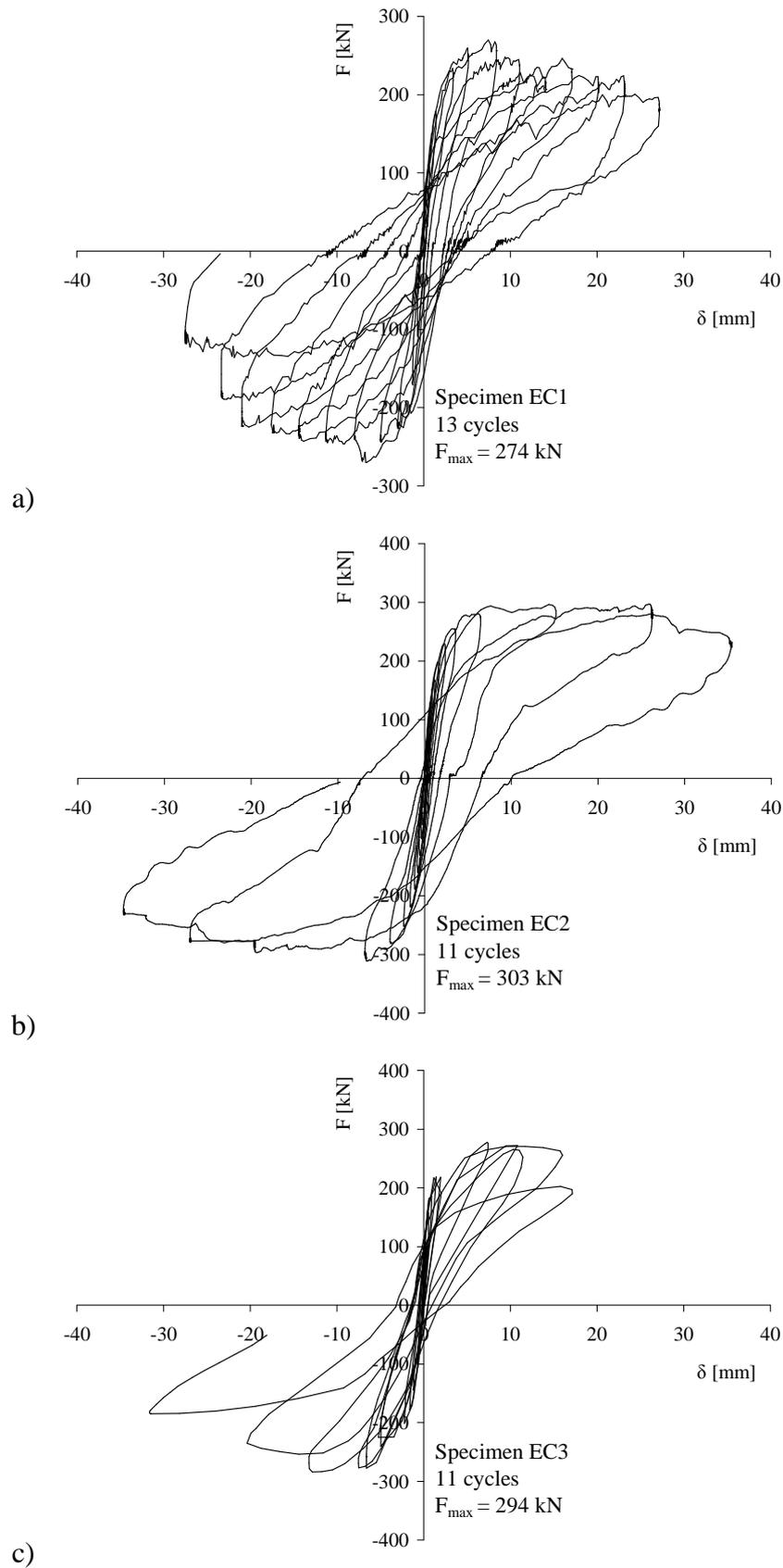
Figure 11: Force vs displacement curves, pumice specimens: a) EC1; b) EC 2; c) EC 3
