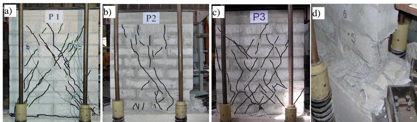
Fig. 12 Cracking patterns of specimens P1 (a), P2 (b), P3 (c) and crushing failure of panel P2(d).
