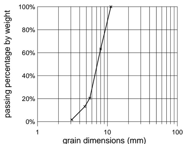
Figure 2: Granulometric curve of pumice grains (3.1-11.2 mm)
