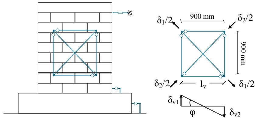
Figure 8: Positioning and gauge lengths of the measuring devices
