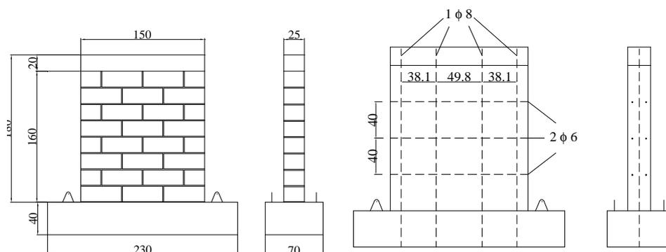
Figure 4: Specimen geometry and reinforcement layout: front and side views
