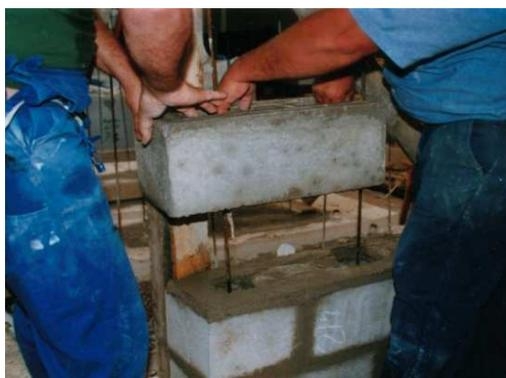
Figure 5: Specimens manufacturing
