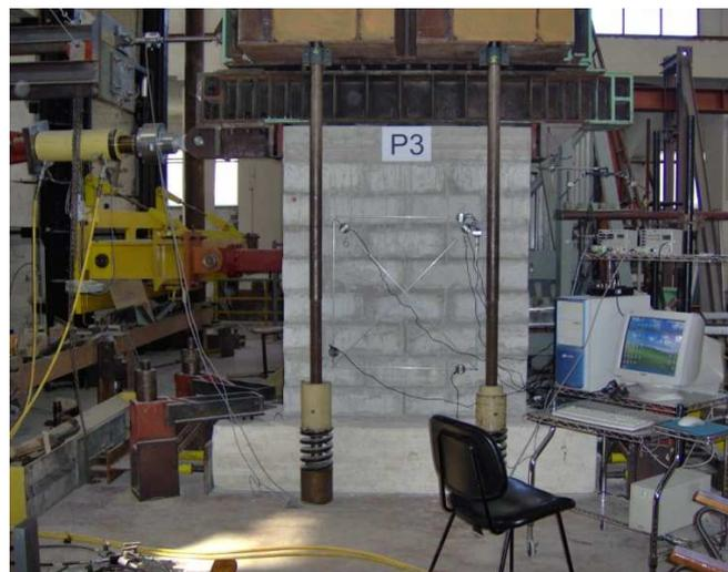
Figure 9: Loading and measuring instrumentation
