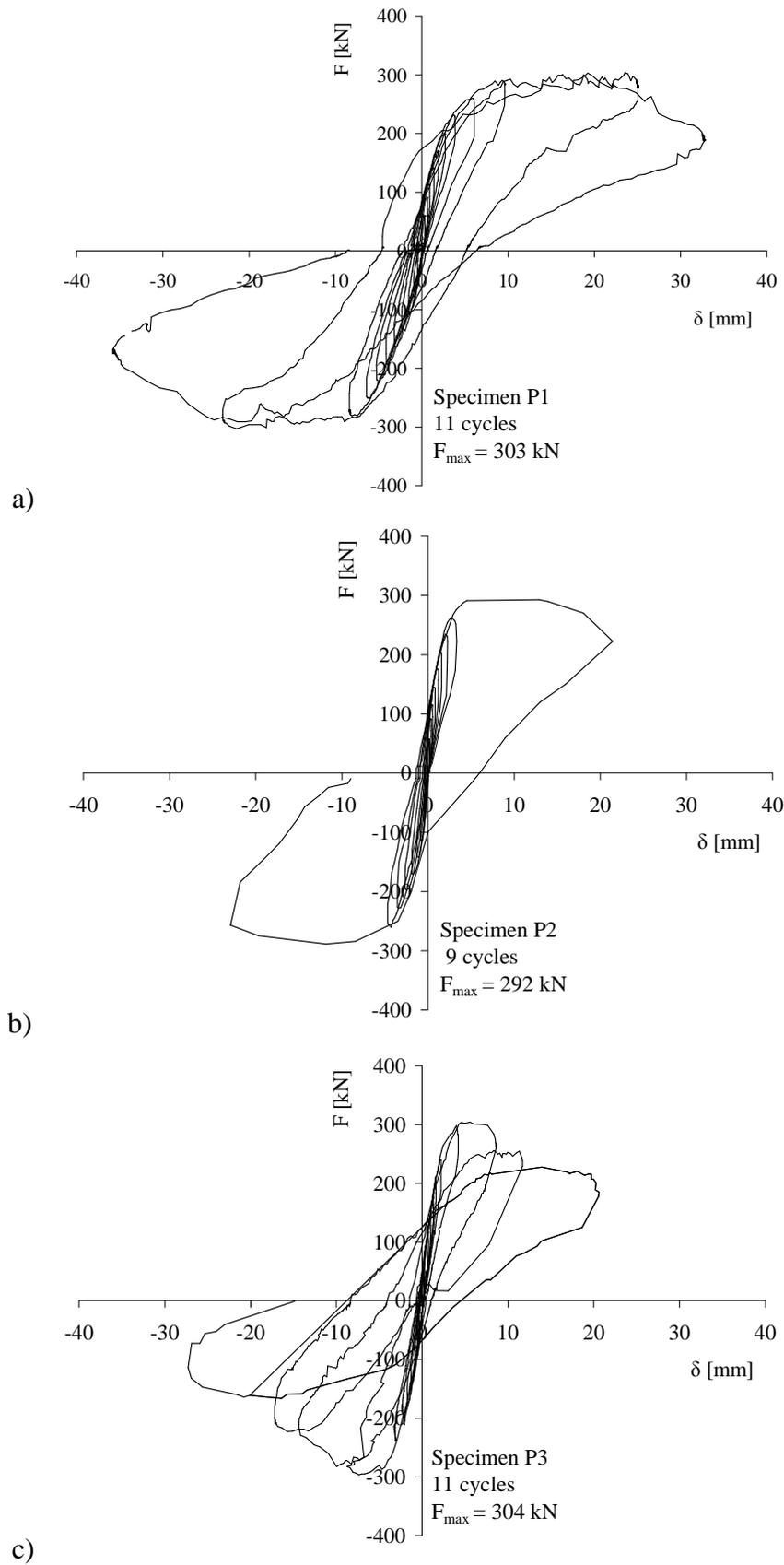
Figure 10: Force vs displacement curves, pumice specimens: a) P1; b) P2; c) P3
