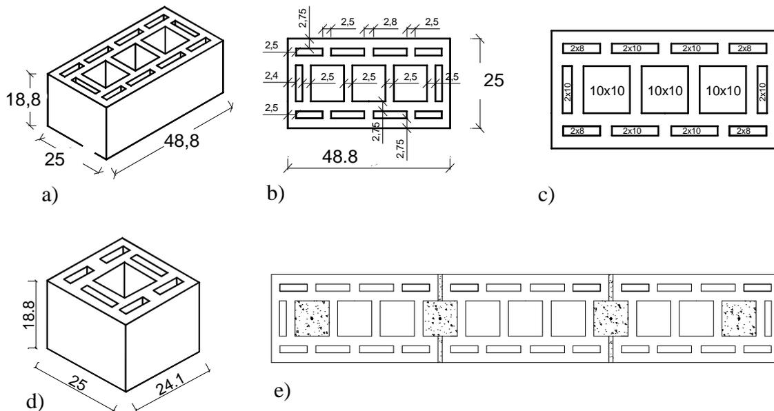
Figure 3: Unit geometry (cm): a) external dimensions; b) tiles dimensions; (c) internal cells; (d) half a block; (e) units arrangement in a course.
