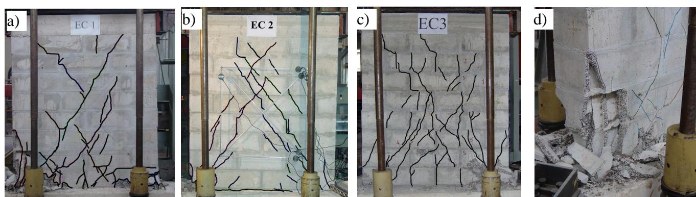
Figure 13: Cracking patterns of specimens EC1 (a), EC2 (b), EC3 (c) and crushing failure of panel EC1(d).
