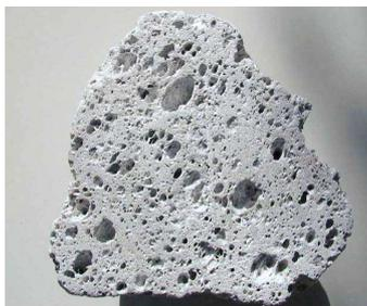
Figure 1: Cross-section of a pumice granule
