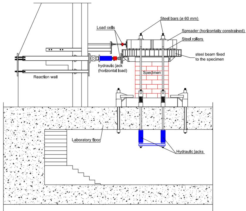
Figure 7: Scheme of the experimental setup and testing frame
