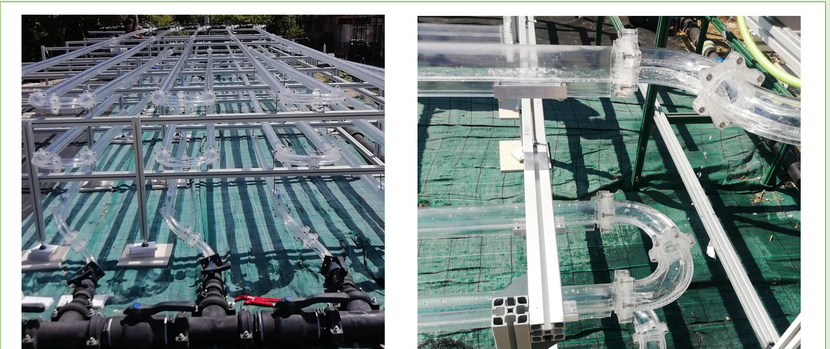
IV. A pilot plant with PMMA tubes was built at UNIPA and autochthonous strains will be cultivated in it
